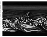
The above microscopic picture of a cross section of FLEXOTHANE® shows how homogenous the PUR coated layer is.
